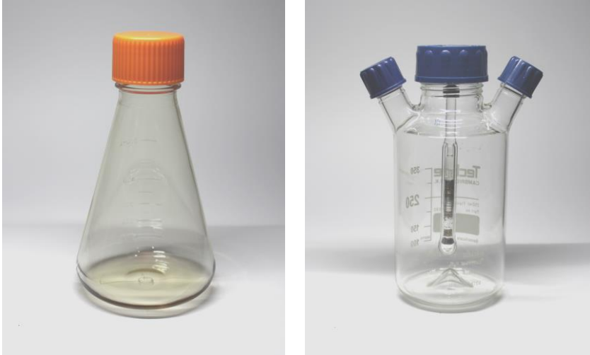
Figure 1. Examples of insect cell culture flasks. (A) Suspension culture shake flask from 125mL to 3L (e.g. Corning™ Erlenmeyer flasks). (B) Suspension culture stirred vessel from 125mL to 1L (e.g. Techne biological stirrers).
