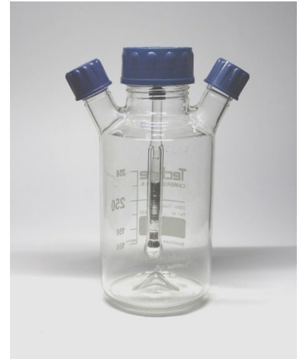
Figure 1. Examples of insect cell culture flasks. (A) Suspension culture shake flask from 125mL to 3L (e.g. Corning™ Erlenmeyer flasks). (B) Suspension culture stirred vessel from 125mL to 1L (e.g. Techne biological stirrers).
